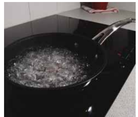
Induction cooktops have a flat, smooth cooking surface that isn't hot to touch when the power is turned on
